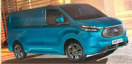
The vehicle has a 74kWh battery combined with an 11kW AC three-phase onboard charger that can fully recharge the battery in 7.8 hours.
