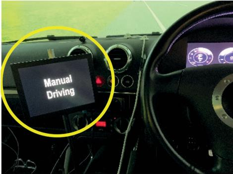
When the vehicle is in manual driving mode, the in-vehicle display screen will show the following visual alert:
